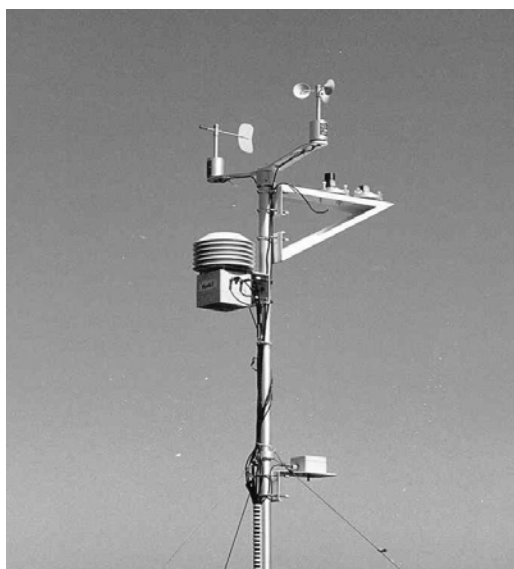
Fig. 7. Automatic meteorological station MiniMet in operation at the Kishinev site
