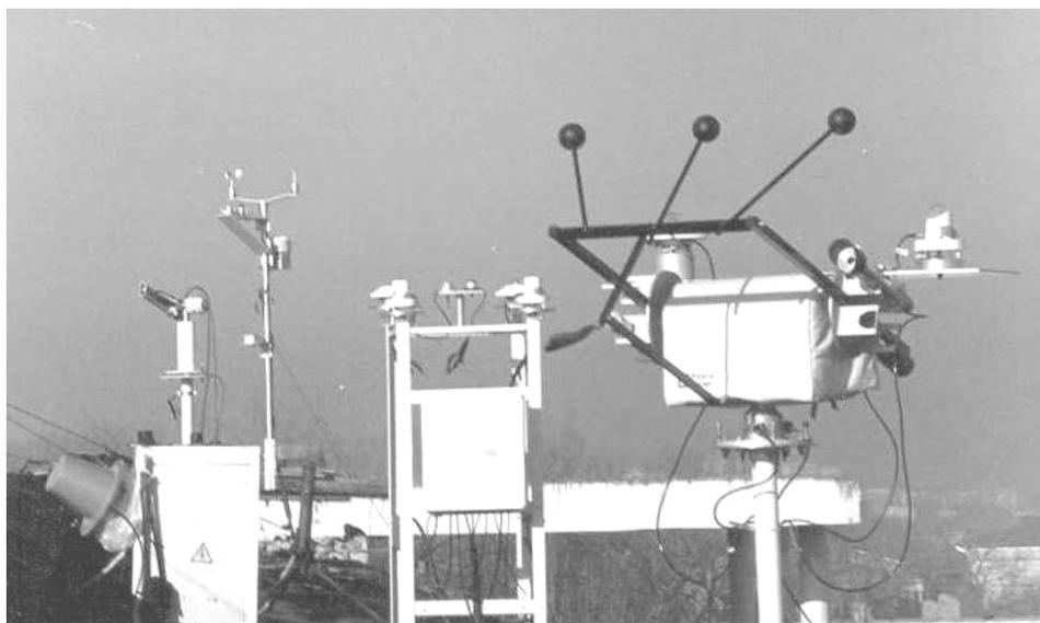
**Fig. 2.** Ground-based multifunctional radiometric complex with operating sunphotometer Cimel CE-318 at the Kishinev site ( $47.0013^{\circ}\text{N}$ ,  $\lambda_o=28.8156^{\circ}\text{E}$ ,  $h=205$  m a.s.l).
