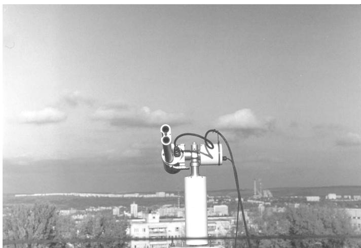
**Fig. 1.** Sunphotometer Cimel CE-318 in operation at the Kishinev site.
